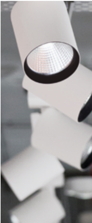
SUPER SPOT 125 I max : 26 630 cd/klm (53 260 cd abs.) FWHM: 2x 3,7°
