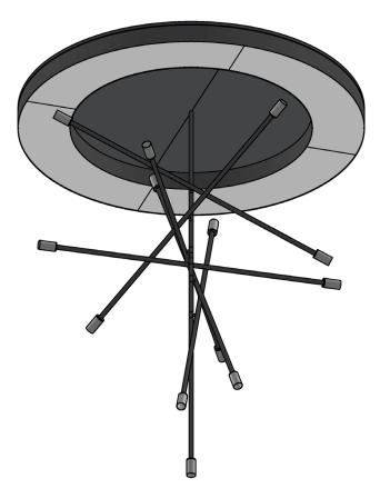
The 10' by 12' custom chandelier features 6 configurable hanging stems, each lit at the ends by cylindrical glass diffusers and a 10' mirrored back ring placed at the top.
