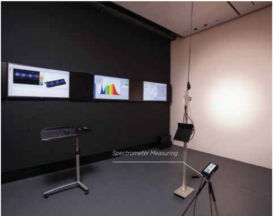
The PROLICHT LIGHT LAB is equipped with a spectrometer, luminance cameras, a heat chamber, a goniophotometer and a 3D printer.
