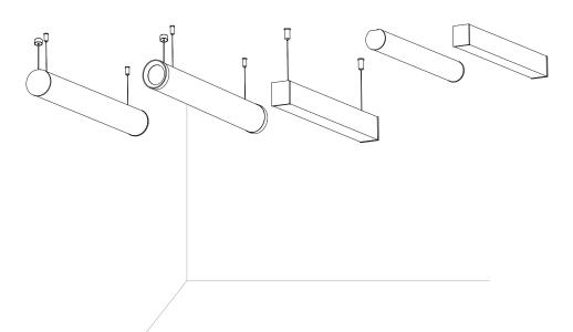
Fino and Bunga are tubular series, offering both surface and suspension applications. Fino features a square design, while Bunga is round. Both models incorporate a satin-finished diffuser, known for its timeless appeal in any setting.
