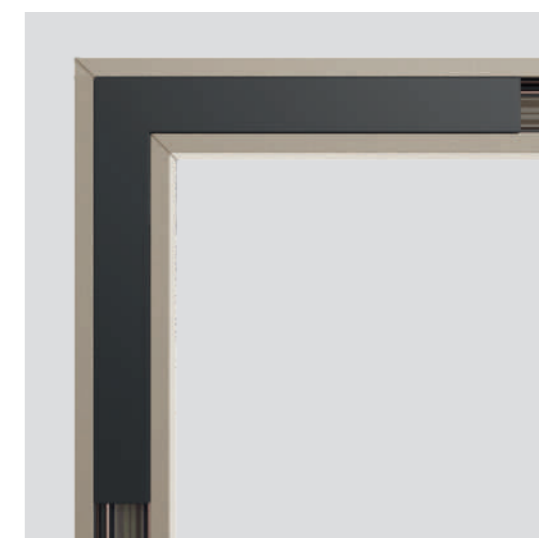
B MITER JOINT The track is designed to be easily cut on site and for a seamless installation of corner elements it is possible to cut the extremities of straight elements at an angle of 45° for a miter-joint connection. If other angles are needed - for a sloping roof for example - the joint can be individualized with a flexible connector.
