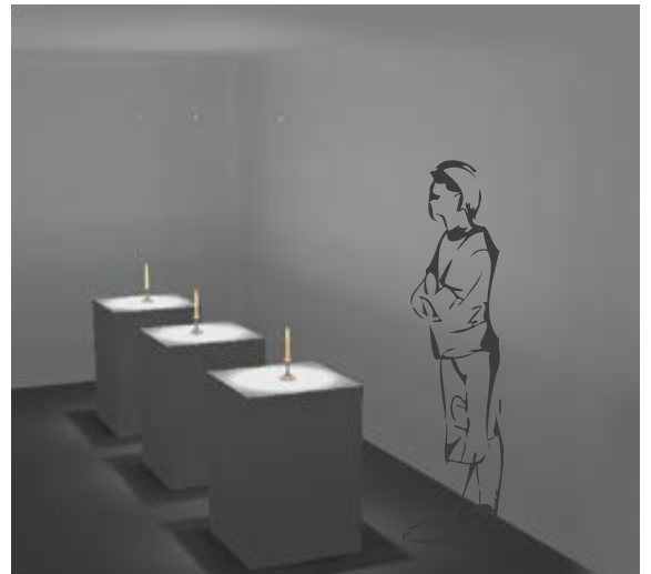
The PROLICHT Super Spots with beam angles under 10° are ideal to illuminate small objects, even from great heights.
