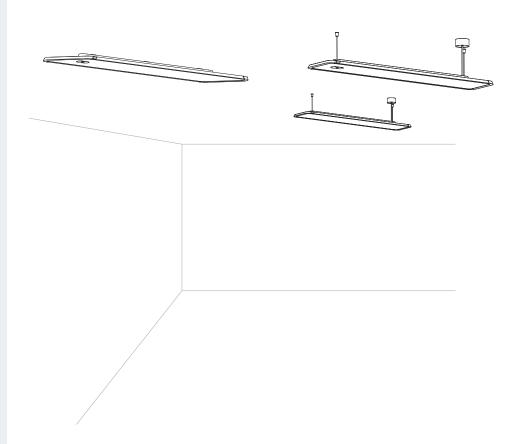
Hadi is a super flat LED luminaire that is designed for office spaces because of it's high efficency at 85%, and UGR of <19.
