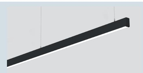
In combination with a white base plate, the white internal reflector creates a perfect mixing chamber. This creates a homogeneous light pattern without individually visible LED dots. All LED boards are protected from electrostatic discharge (ESD) and direct contact with the LED by a highly transparent acrylic glass.
