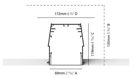
A: Opening width | B: Recess depth | C: Profile height D: Width including mounting brackets
