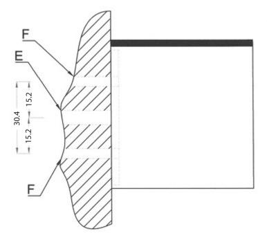
E : Cable entry F : Wall plug G: Wall Bracket
