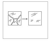
If diffuser is damaged, replace before powering on the fixture.
