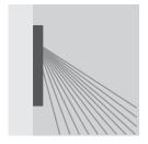
A high luminous efficiency diffusing methacrylate lens with a very broad beam both transversely and longitudinally.
